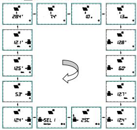
Echo Loop: PV voltage ——PV current ——PV power——Battery power—
