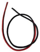
**Step 2:**Strip one end of the copper wire connected to the rocker switch for about 15mm.
