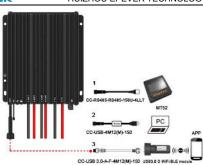
Note: Only the Tracer-CPN series support the external Bluetooth module, the Tracer-CPN (BLE) series has a built-in Bluetooth module. MT52 is not waterproof. If used outdoors, please ensure proper waterproofing and dust protection. And MT52 cannot set the relevant parameters of the lithium battery and load mode.
