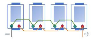
WARNING: When the batteries are connected in series or parallel, measure the battery voltage with a multimeter. The battery voltage shall be consistent or the voltage difference is less than 0.2V (it is normal if there is a slight spark during the parallel connection). It is forbidden to connect the battery in series/parallel when the battery voltage exceeds this range.
