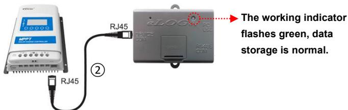
Note: eLOG01-S-G3 data storage interval defaults to 900 seconds, and eLOG01-M-G3 data storage interval defaults to 15 minutes. The same module can record a maximum of 20,000 data entries.
