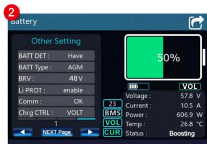
On the home screen, touch
