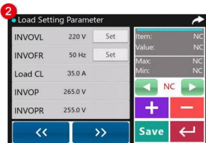
On the parameter setting screen, click **Load** to enter the load parameter setting screen. The following information is displayed:
