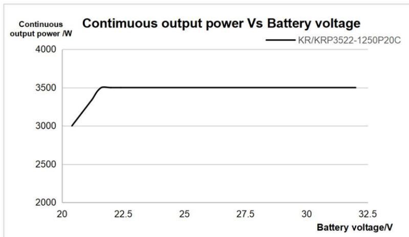
The parameters are measured in the condition of 48V/25 °C.
