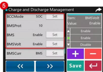
5. Click **>>** to switch to the "Charge and Discharge Management" interface and set "BCCMode (Battery Charging Control Mode), BMSProt (BMS Protocol), BMS (BMS Enable), and BMSVolt (BMS Voltage Control)." After the settings are complete, click **Save** to issue new parameter value.
