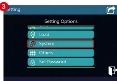
3. Slide up and down on the current screen, and click **System** to enter the system parameter setting screen.
