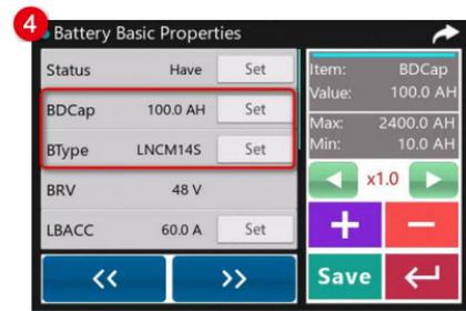
4. Depending on the battery actually used, set "BDCap (Battery Design Capacity) and BType (Battery Type)". After the settings are complete, click  to issue new parameter value.
