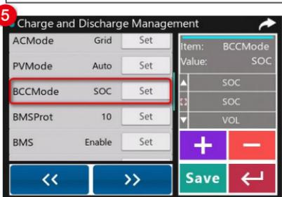
5. Click **>>** to switch to the "Charge and Discharge Management" screen, and set "BCCMode (Battery Charging Control Mode)" to "VOL" or "SOC." After the settings are complete, click **Save** to issue new parameter value.
