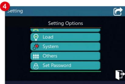
The parameter setting screen includes: PV (PV parameter setting), Charge (battery charge control parameter setting), Grid (Grid parameter setting), Load (Load parameter setting), System (System parameter setting), Others (Other parameters setting) and password setting.
