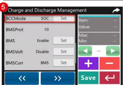
5. Click **>>** to switch to the "Charge and Discharge Management" screen and set "BCCMode (Battery Charging Control Mode)." After the settings are complete, click **Save** to issue new parameters.
