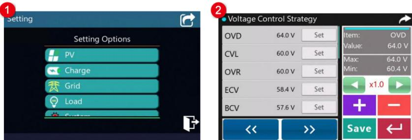
On the parameter setting screen, click **Charge** to enter the battery charge control parameter setting screen. The following information is displayed:
