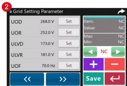
On the parameter setting screen, click **Grid** to enter the grid parameter setting screen. The following information is displayed:
