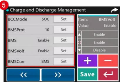
5. Click **>>** to switch to the "Charge and Discharge Management" interface and set "BCCMode (Battery Charging Control Mode), BMSProt (BMS Protocol), BMS (BMS Enable), BMSVolt (BMS Voltage Control), BMSCurr (BMS Current Control)." After the settings are complete, click **Save** to issue new parameters.
