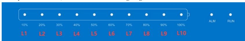
② A total of 12 LED lights on the light board, each light can display red, yellow, blue, green and other colors. It is divided into 3 categories according to the use of the light:
