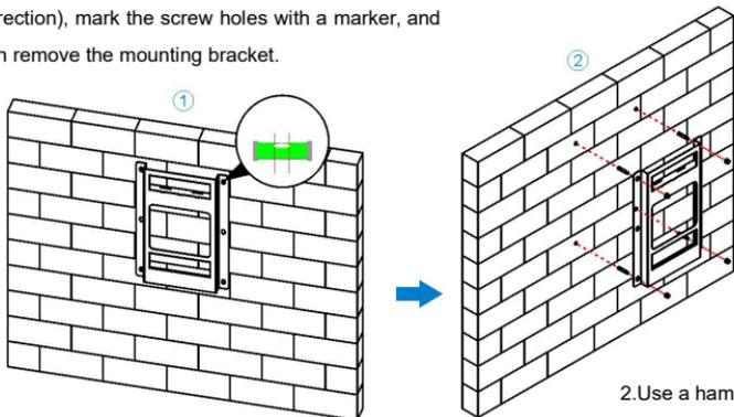
2. Use a hammer drill to drill a hole in the wall (diameter: 10mm, depth: 65mm), insert the M8 expansion screw and tighten it.
