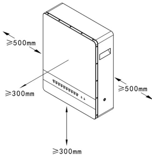
The left and right distance between battery packs is recommended. Minimize the distance as much as possible.
