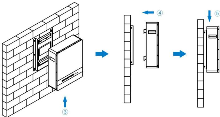
3. Lift the lithium battery vertically and align it with the mounting bracket slots.
